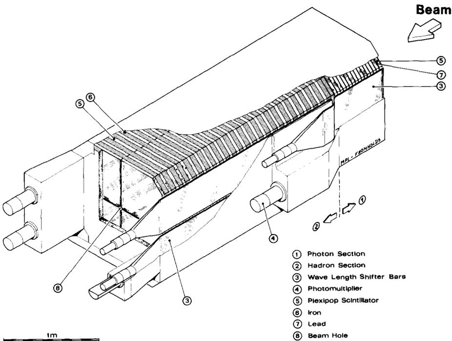
Fig. 12. Perspective view of the downstream calorimeter.
