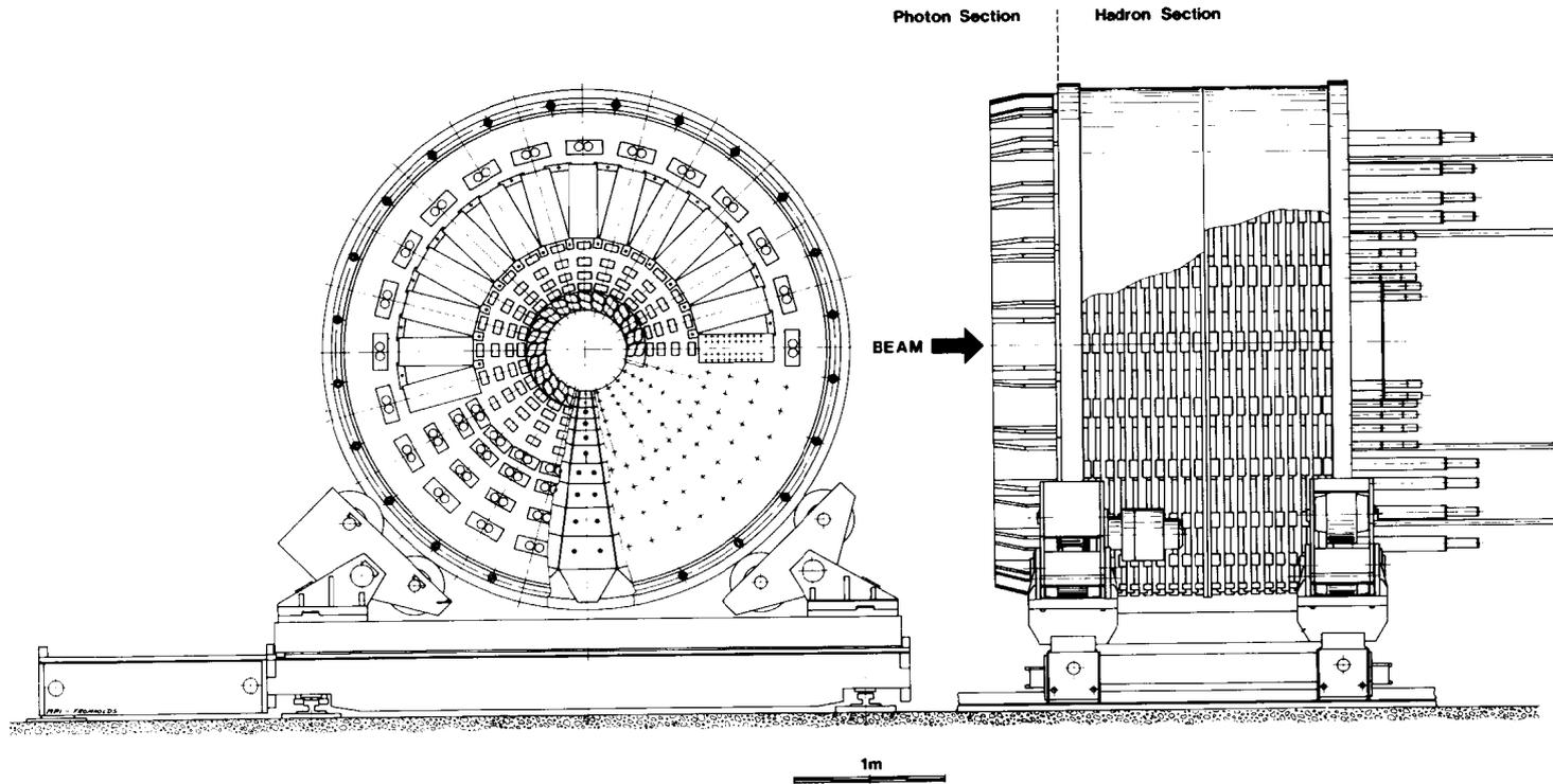
Fig. 1. Front and side view of the ring calorimeter and its support structure. Indicated is one of the 24 sectors of the calorimeter, which is subdivided into 10 individual cells. The photomultipliers are mounted at the downstream end of the calorimeter.
