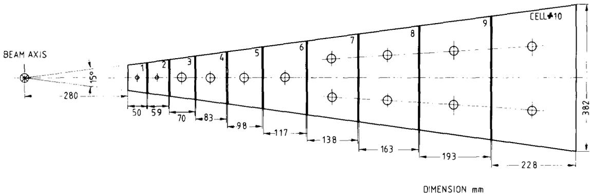
Fig. 2. One of the 24 sectors, which is subdivided into 10 individual cells, is illustrated. Dimensions are in mm.
