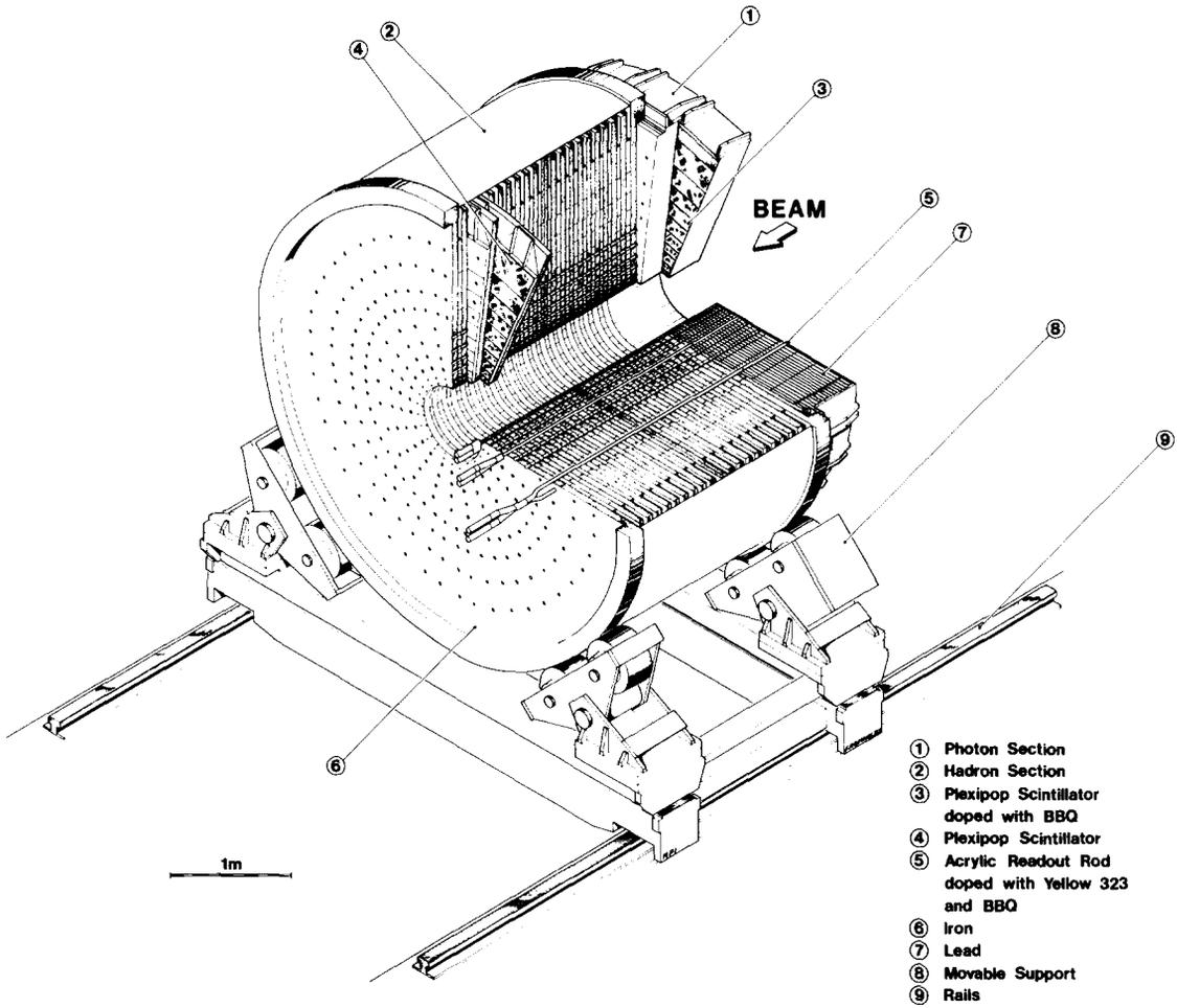
Fig. 5. Perspective view of the ring calorimeter.
