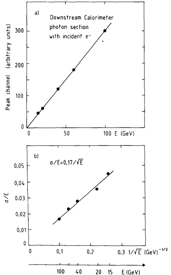
Fig. 13. (a) The peak pulse height as a function of the incident electron energy and (b) the energy resolutions  $\sigma/E$  are shown for the photon section of the calorimeter.
