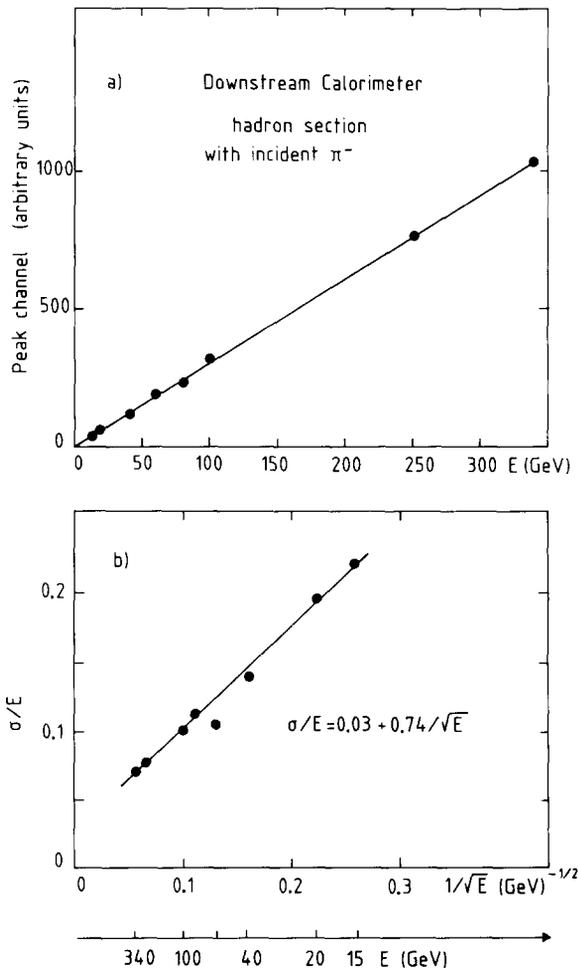
Fig. 14. (a) The peak pulse height as a function of the incident pion energy and (b) the energy resolutions  $\sigma/E$  are shown adding the information of the photon and hadron section as described in the text.
