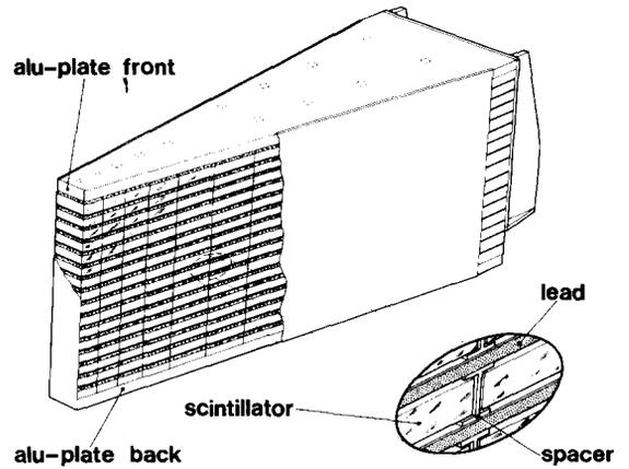
Fig. 7. Perspective view of one of the photon calorimeter sectors.
