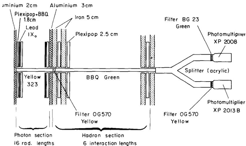
Fig. 3. The principle of the two coloured wavelength shifter optical readout system is illustrated.
