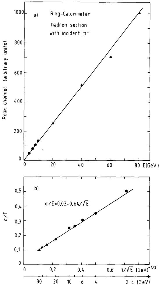
Fig. 9. (a) The peak pulse height as a function of the incident pion energy and (b) the energy resolutions  $\sigma/E$  are shown adding the information of the photon and hadron section as described in the text. The triangles and the points are the results obtained with the ring and the test calorimeter respectively.
