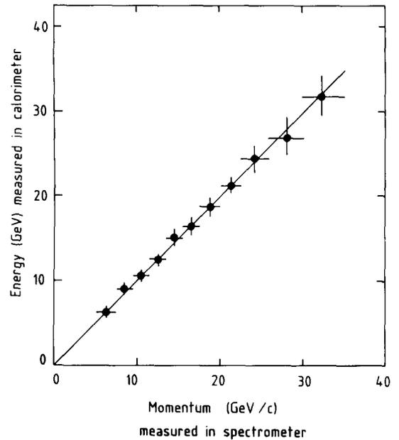
Fig. 10. Energy deposited in the calorimeter vs the momentum measured in the spectrometer for charged particles assuming they are pions. The error bars on the ordinate represent the precision of determining the peak pulse height. The error bars on the abscissa represent the bin size.
