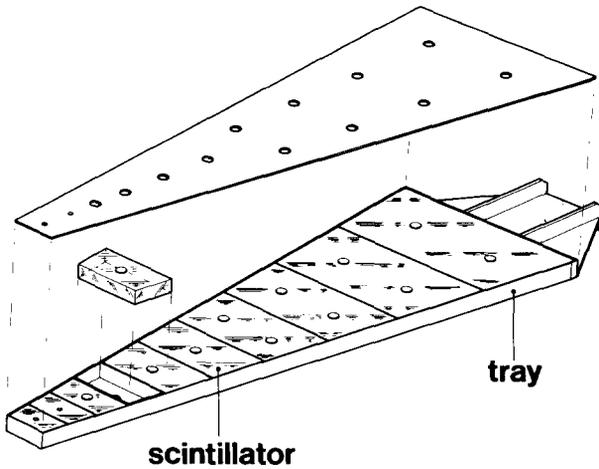
Fig. 6. One of the plastic trays with scintillators inside.
