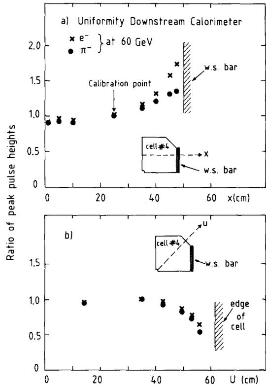
Fig. 15. The ratio of the peaks of the pulse height distributions measured along (a) the x- and (b) the u-axis respectively to that measured at the calibration point. The scan was performed with the incident beam travelling parallel to the calorimeter axis.
