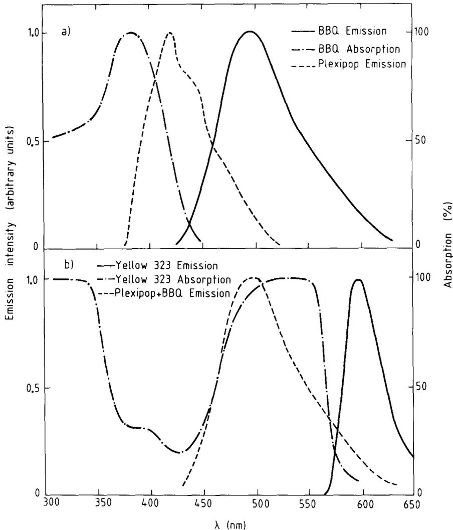
Fig. 4. The emission spectra of the scintillator materials and the emission and absorption spectra for the wavelength shifter rods are shown (a) for the hadron section and (b) for the photon section of the calorimeter. All emission spectra were supplied by Röhme GmbH in Darmstadt, W. Germany.
