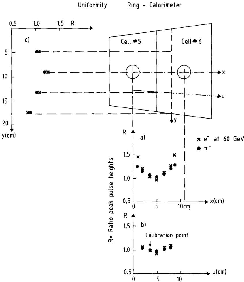
Fig. 11. The ratio of the peak of the pulse height distributions measured along (a) the  $x$ -, (b) the  $u$ - and (c) the  $y$ -axis respectively to that measured at the calibration point. The scan was performed with the incident beam travelling parallel to the readout rods.
