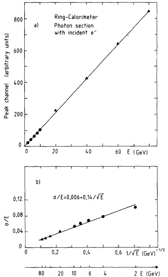
Fig. 8. (a) The peak pulse height as a function of the incident electron energy and (b) the energy resolutions  $\sigma/E$  are shown for the photon section of the calorimeter. The triangles and the points are the results obtained with the ring and the test calorimeter respectively.
